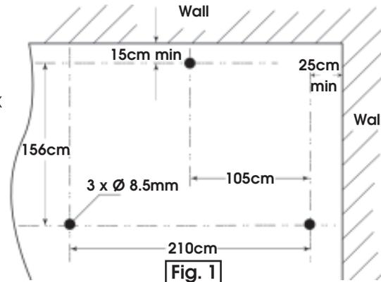
1. Choose suitable location, taking into consideration the operation, i.e. the X & Y-axis, allow sufficient clearance especially on the right hand side of the machine to enable unhindered use of the handwheel etc.
