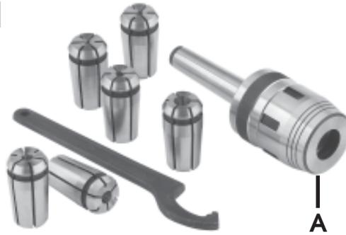
1. Insert the shank of the chuck into the Mill Head Spindle and screw on to the end of the draw bolt, shown in Fig 7, page 18. Tighten the draw bolt, holding the spindle steady by hand or by using a tommy bar (not provided) in the hole provided in the spindle.
